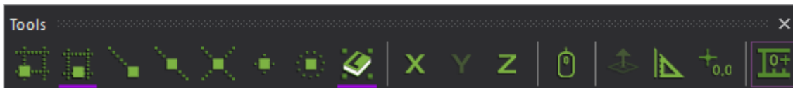
Figure 9 - Tools toolbar offers two new Snaps, Mid-Grid (2nd button), and Library Snap (8th button).
